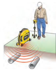
Induce a signal to locate utilities.
