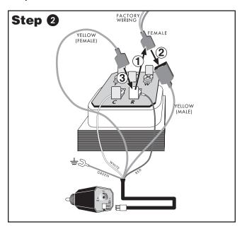
① Unplug the factory-wired quick connect from terminal **R** and ② plug into YELLOW wire with *male* connector. ③ Plug YELLOW wire with *female* connector into terminal **R**.
