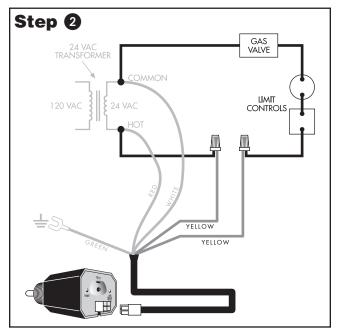
Cut-off the connectors and strip the ends of the two yellow wires of the Model 1100 harness. Break into the burner circuit between the *hot* side of the transformer (R) and other limit controls. Connect either YELLOW wire to the *hot* side. Connect the other YELLOW wire in series with other limit controls.
