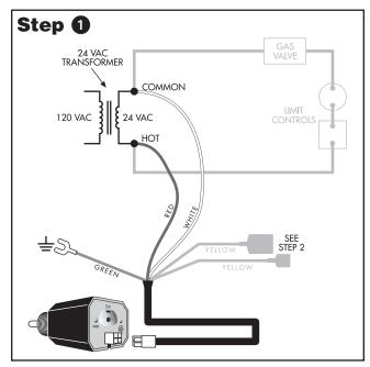
Connect RED wire to *hot* side of 24 Volt boiler transformer **(R)**. Connect WHITE wire to common side of 24 Volt boiler transformer **(C)**. Connect the GREEN wire to any suitable, unpainted ground screw.
