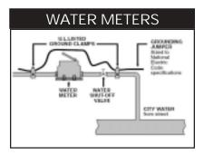
GROUNDING CLAMPS ONLY FOR WATER PIPE
