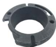
Problem: Broken Flange Solution: 3-D encapsulation
