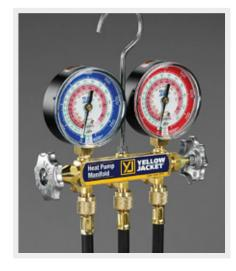
The YELLOW JACKET® Heat Pump Manifold features two 800 psi gauges to read all heat pump pressure conditions. Traditional lo-side manifold gauges can be susceptible to damage when heat pumps go into heating mode. Because the lo-side gauge of the YELLOW JACKET Heat Pump Manifold is also designed for pressures up to 800 psi, it can read the pressure whether the pump is in heating mode, cooling mode or transition.
