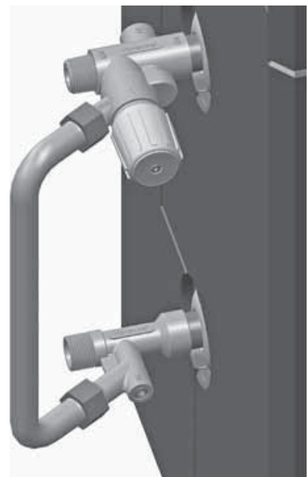
Figure 5 Mixing valve assembly, Aqua Logic (CWH) rotated, connections on left
