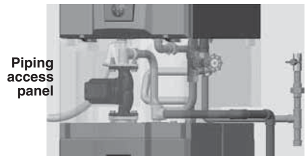
Figure 3 Align water heater under boiler as needed for the piping access panel to fit in place
