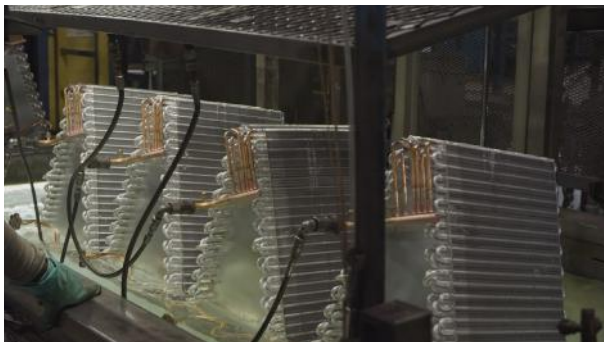
AIR UNDER WATER TESTING
