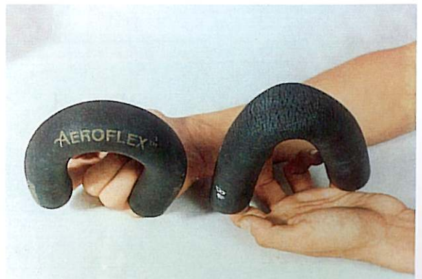
Two years exposed to sun light experiment proves that Aeroflex has outstanding ultraviolet and weather resistance. The service life under normal condition for hot water pipe is estimated to be more than 10 years.
