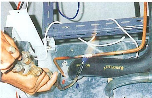
Self-extinguishing property low smoke density and non-melting characteristic while burning make Aeroflex widely used in air-conditioning systems.
