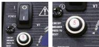
Protected switches & circuit breaker
