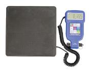
Using the Latest Technology, the PCS220 Makes Charging a System Fast and Reliable. Just Set the Desired Amount of Refrigerant to Charge the System and the Built-In Solenoid Delivers the Precise Weight, then Sounds the Alarm Signaling the Completed Job.
