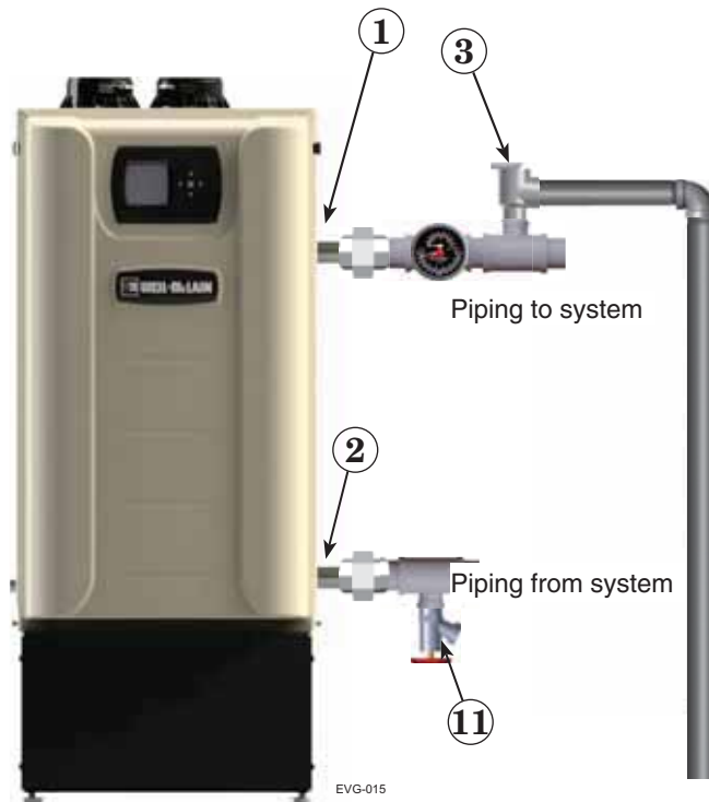
Figure 8 Install pipe fittings for relief valve and pressure/temperature gauge — DO NOT mount relief valve until AFTER hydrostatic testing (see legend below)
