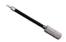
With its flexible shaft, it allows the service technician to easily access valve cores that may be blocked . The center section of the tool has a slip fit design to allow the user to hold and spin the knurled end to loosen or tighten the valve.
