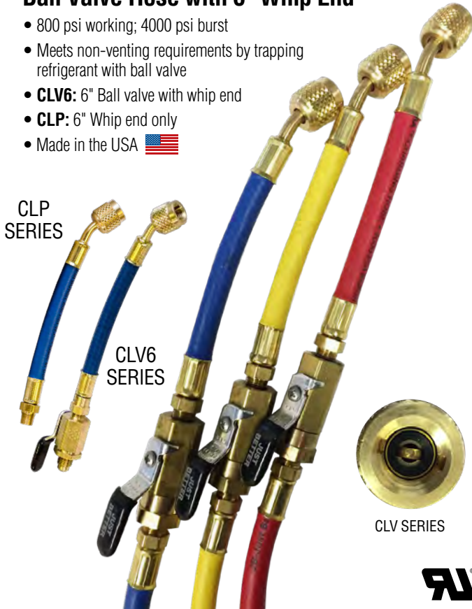
CLV SERIES KOBRA® 1/4" X 1/4" W/BALL VALVE WHIP END (PSI 800/4000)
