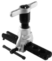
T30600 Ratcheting eccentric cone flaring tool with internal clutch to prevent over-torquing. For tube OD: 3/16", 1/4", 5/16", 3/8", 1/2", 5/8", 3/4"
