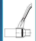
3. Heat the tube and coupling, applying heat to all the parts.
