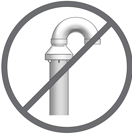
Figure 5-5 Do Not Install U-Bend to Rain Cap
