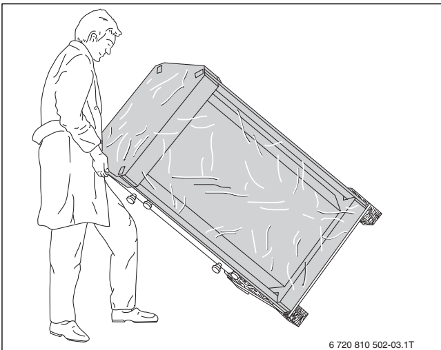
Fig. 8 Positioning the tank
