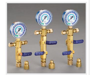
SUPEREVAC® manifolds are engineered as system components for the SUPEREvac® pumps to help decrease vacuum time by over 50 percent and improve micron readings. Mounts with 1/2" or 3/8" Female flare quick coupler and provides easy connections for two 3/8" vacuum hoses.
