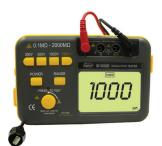
The Versatile M1000D Provides the User Selectable Test Voltage Ranges of 250V/500V/1000V to Test Insulation Resistance and Can Also be Used to Measure AC Voltage up to 750AC.
