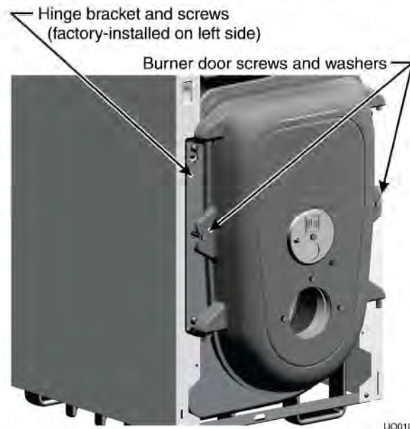
Figure 4 Burner door hinge installation
