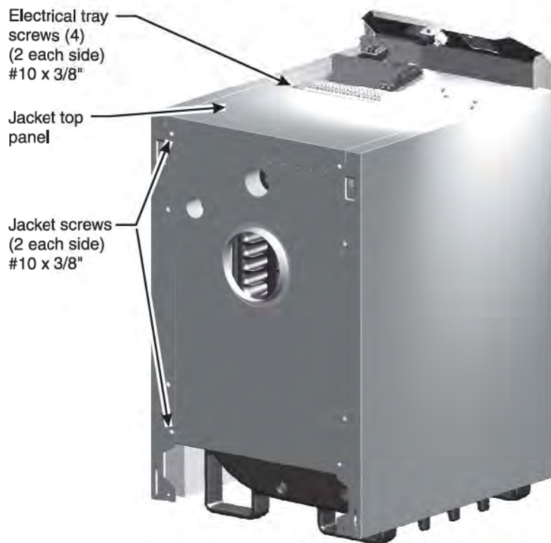
Figure 20 Jacket components and hardware
