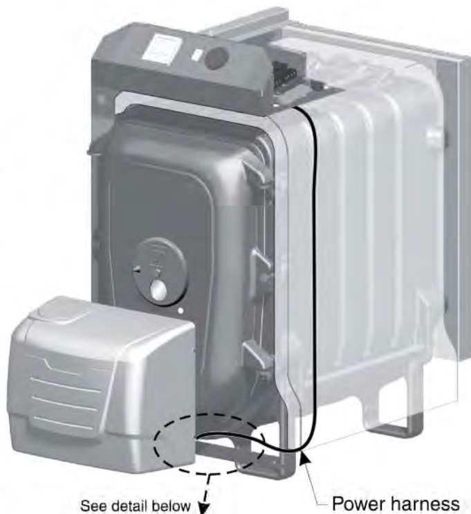
Figure 14 Burner harness routing
