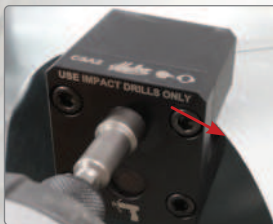
Begin crimping at angle
