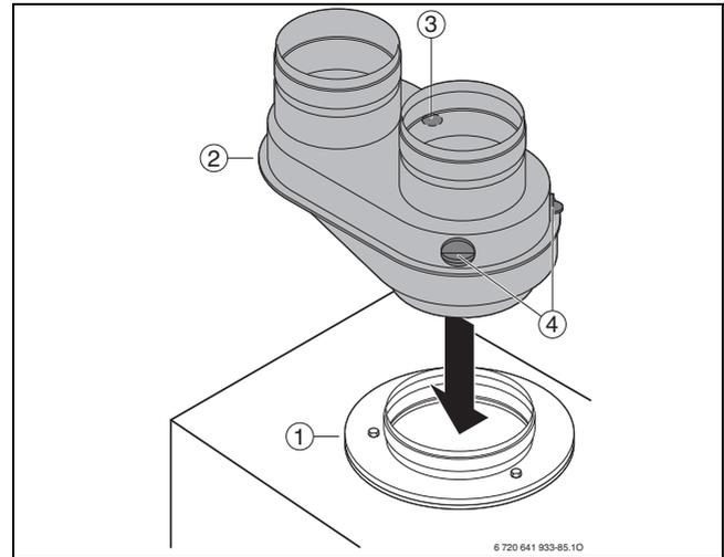
Fig. 27 Flue gas adapter
