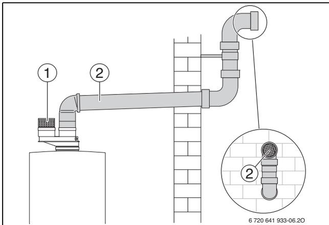
Fig. 32 Horizontal venting system (room air only)
