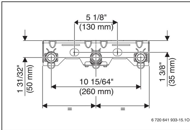
Fig. 19 Hydraulics connection plate for heating boiler ZBR...-3A (top view)
