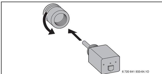
Fig. 24 Installing a LWCO device - LWCO adapter
