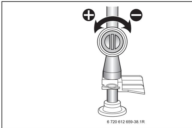
Fig. 78 Set CO<sub>2</sub> or O<sub>2</sub> level for maximum nominal output
