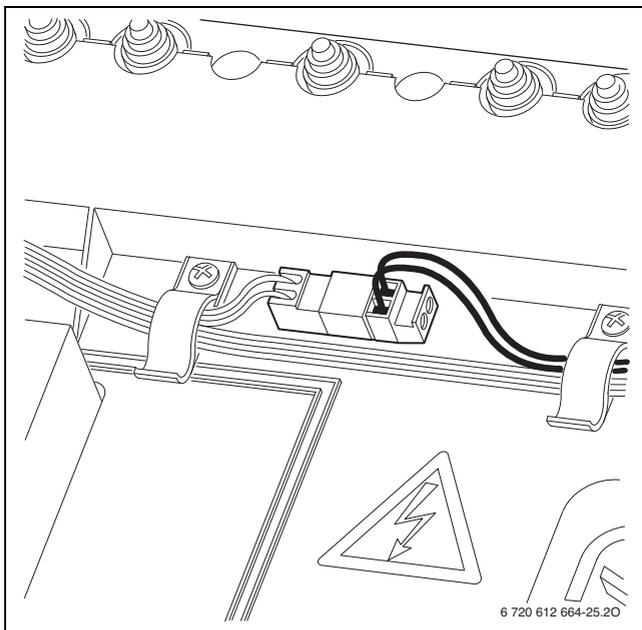
Fig. 51 Electrical wiring of external supply temperature sensor
