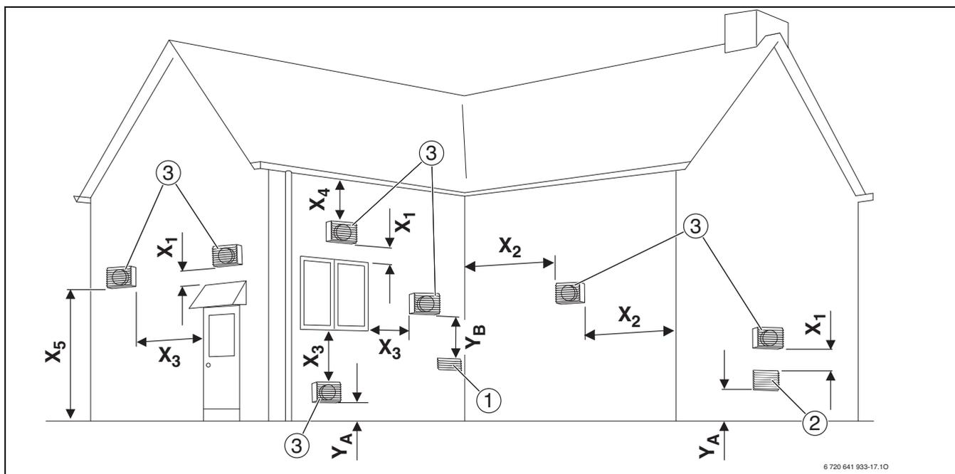
Fig. 31 Vent and combustion air pipe position
