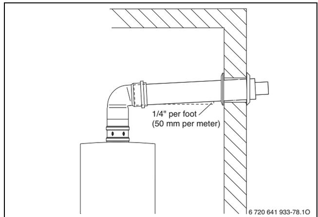
Fig. 41 Horizontal venting system (telescopic concentric vent kit)
