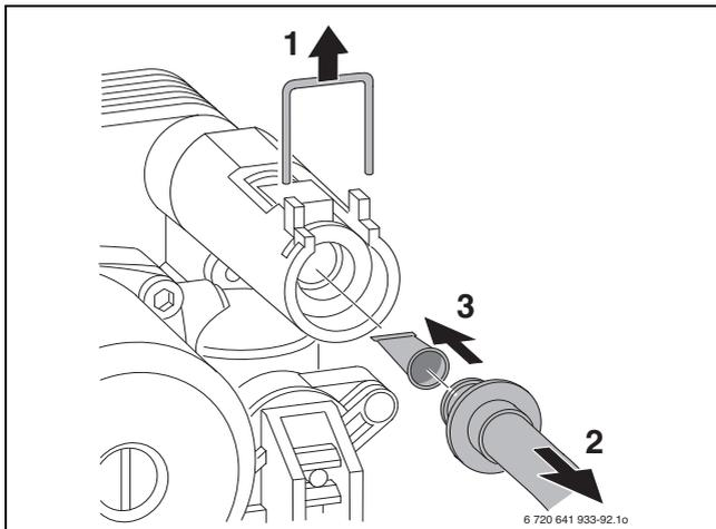
Fig. 83 Filter in fresh water pipe
