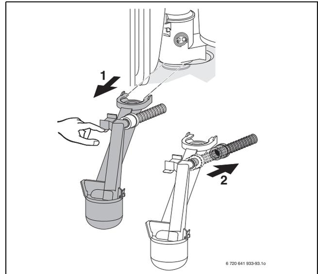
Fig. 98 Removing the condensate trap
