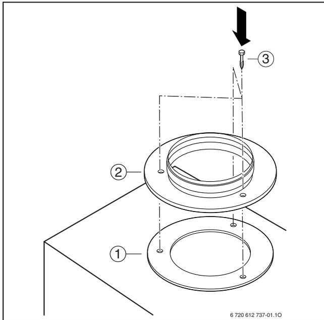
Fig. 26 Attaching the vent flange and gasket
