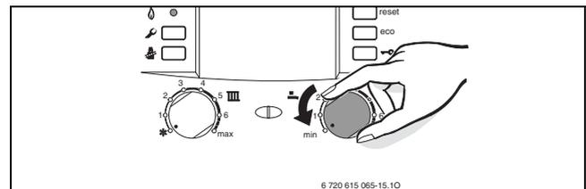
Fig. 70 Frost protection for the DHW tank
