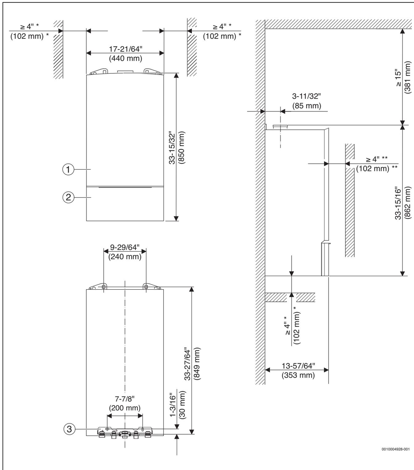
Fig. 4 Dimensions and minimum clearances (front view, rear view, side view)
