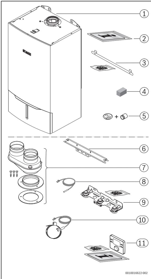
Fig. 1 Scope of delivery heating boiler ZBR...-3A
