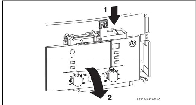
Fig. 42 Fold the Heatronic down
