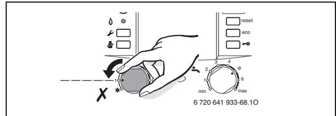
Fig. 69 Frost protection of the heating system
