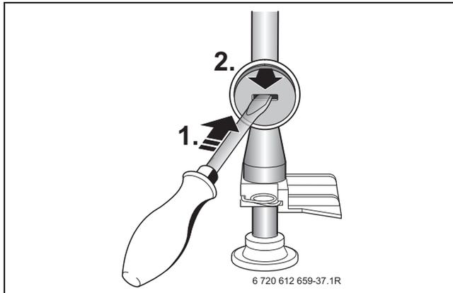
Fig. 77 Remove seal from the gas throttle
