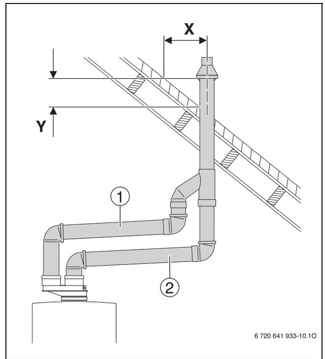
Fig. 38 Vertical venting system (sealed combustion)
