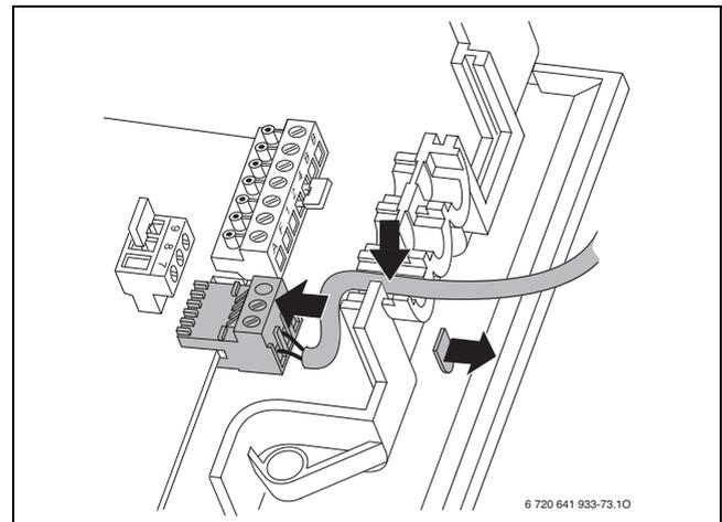
Fig. 47 Electrical connections DHW tank temperature sensor
