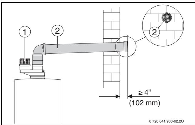
Fig. 33 Horizontal venting system (room air only)
