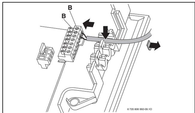
Fig. 44 Electrical wiring BUS-cable at the boiler
